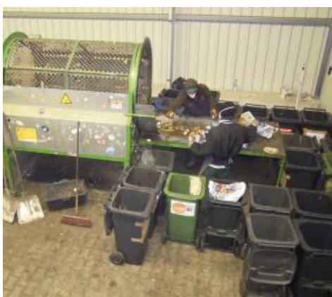
F-03: Sorting via small mobile drum screen
