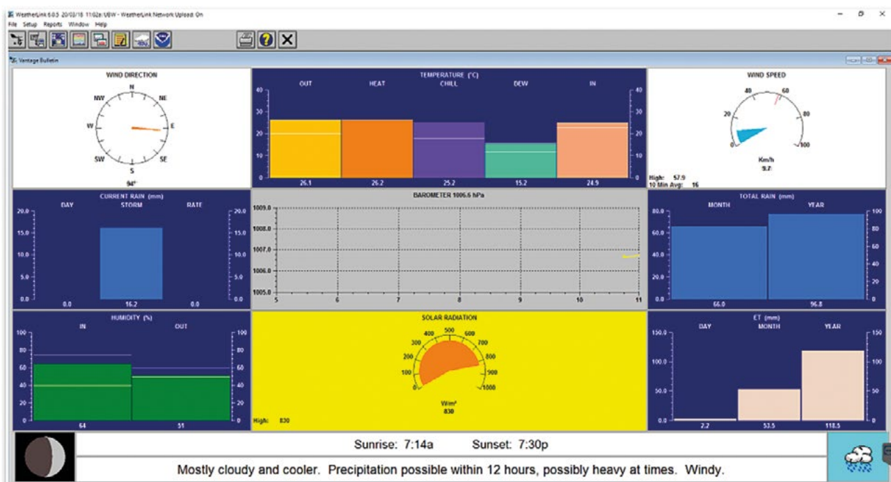
Figure 40: Minigrid weather station dashboard – Display of the DAVIS Weather Link Dashboard
