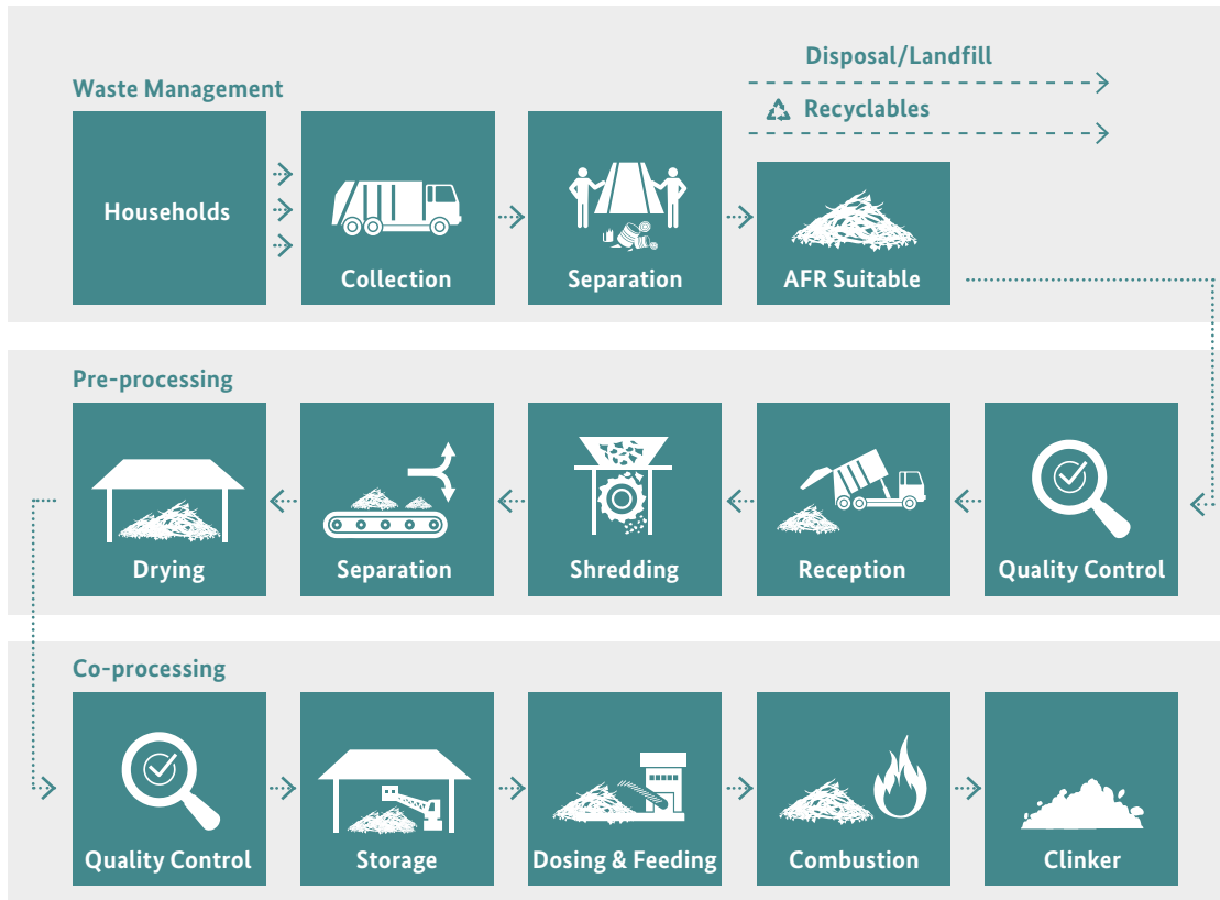
Figure 5: Integration of pre- and co-processing in a MSW management concept.
