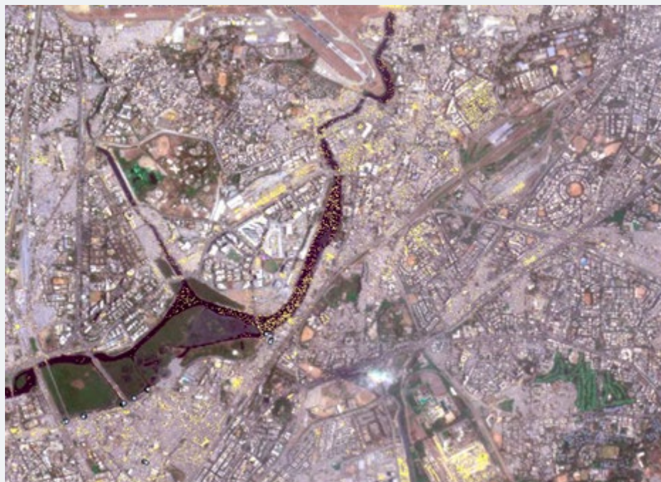
Figure 11: A cropped image (RGB) from Planet 3-m data for Mumbai showing the potential waste-positive localities after applying heuristic feature space reduction and clustering. Yellow pixels represent plastic waste locations obtained from the preliminary analysis.
