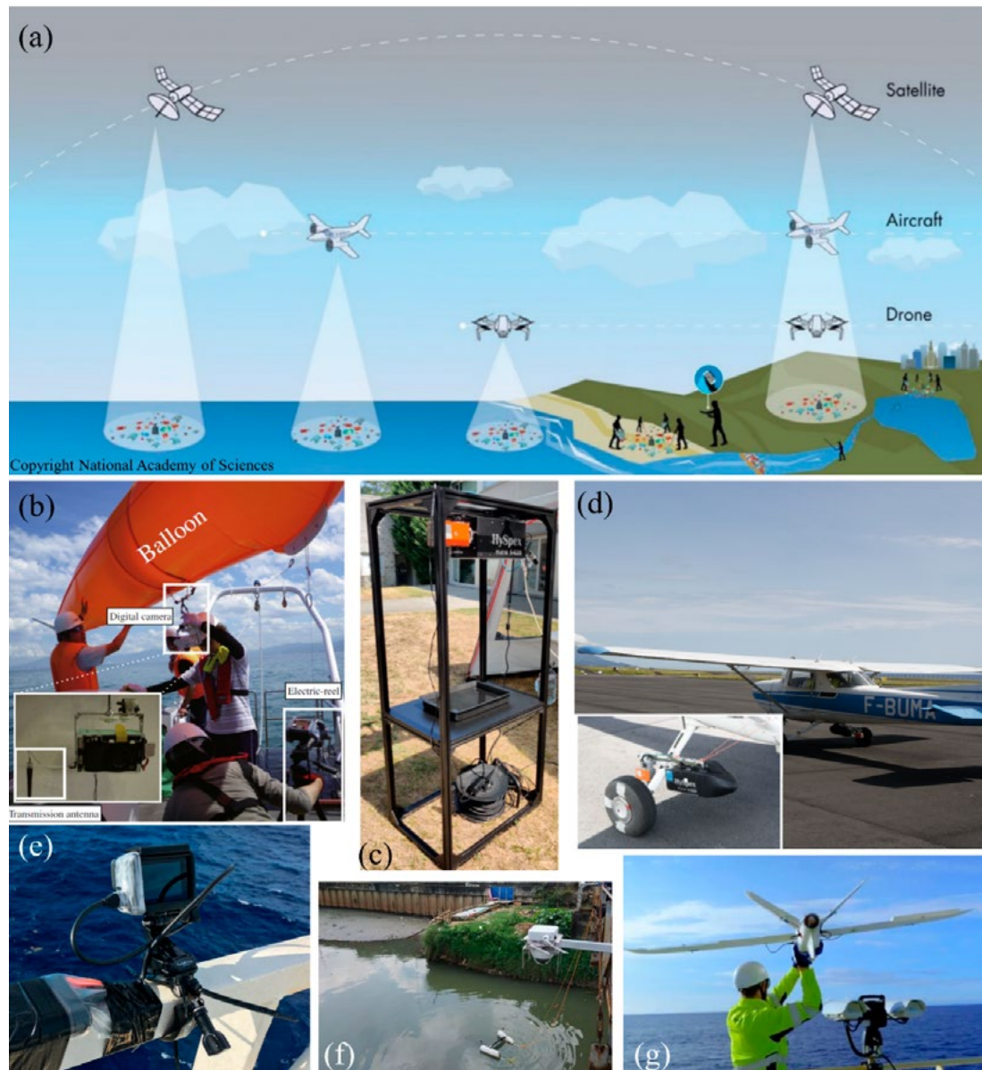
Figure 5: Overview of remote sensing platforms relevant for plastic waste 65 , examples from (a) experiments over water using sensors (b) attached to balloons 49 , (c-d) on moveable frames and aircrafts 46 , (e) fixe to ships 33 , (f) fixed on bridges and (g) on drones 33 .
