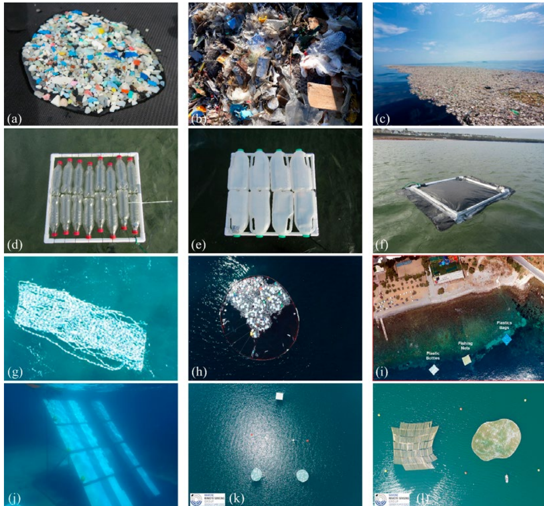
Figure 4: Examples of plastic samples of varying sizes that have been observed in remote sensing experiments (a) ocean harvested microplastics 35 , (b) soup of plastics in the Port of Antwerp 40 , (c) mixture of litter in windrows imaged by Caroline Power, (d-f) 0.5 × 0.5 m aggregated plastic bottles and sheets 34 , (g) 3 × 10 m target of floating plastic bottles 37 and (h-l) large floating and submerged plastic structures. (Images provided by Konstantinos Topouzelis).
