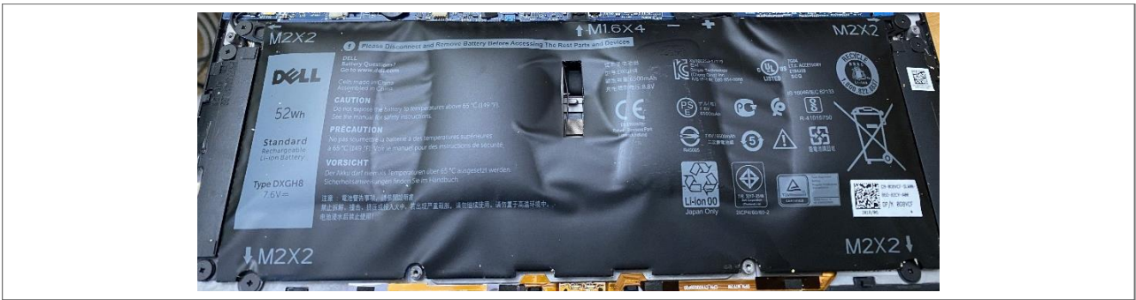
Figure 4-4: Swollen pouch cell battery
