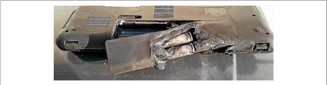
Figure 4-3: Damaged cylindrical cell battery
