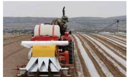
A farmer is applying the PE mulch film on the test field in Gansu province. Photo: © GIZ/Jingyue Hou
