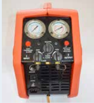
Figure A: Commonly used portable recovery unit for refrigerant extraction (left: side view, right: front view). This unit does not contain a built-in oil separator.
