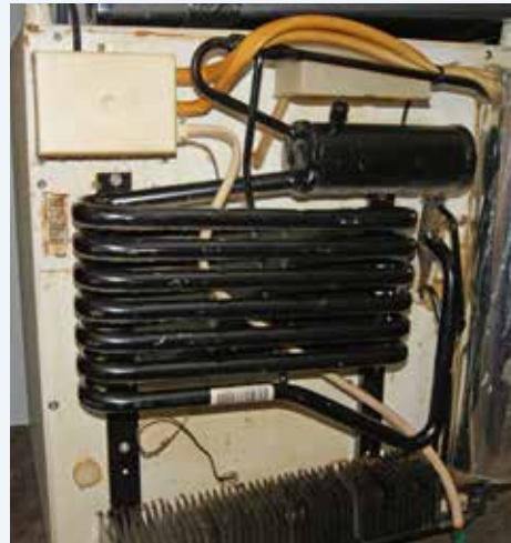
Figure 4: Refrigerator that uses ammonia as refrigerant. The condensing unit (cooling coil) is much coarser compared to refrigerators that use halogenated refrigerants or butane.
