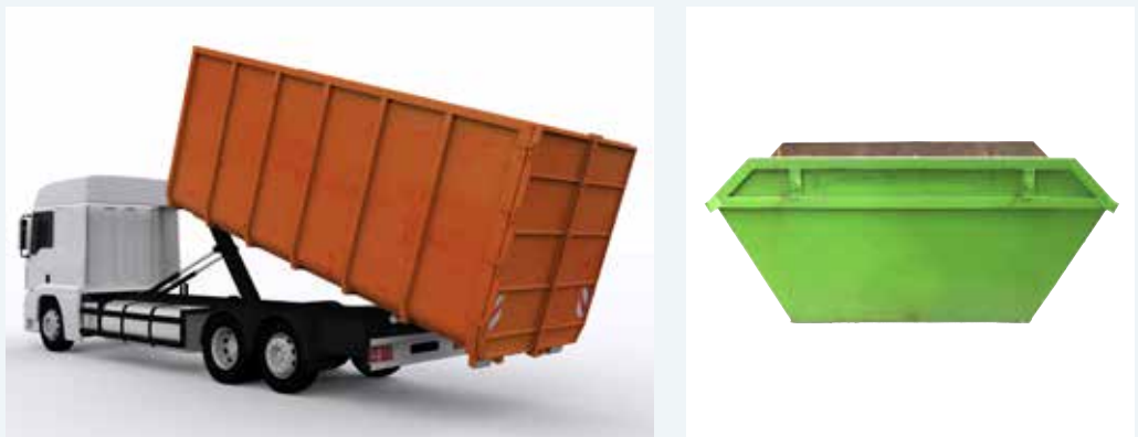
Figure 16: Roller container (left) and smaller 7 m 3 skip (right) for the transport of WEEE and recovered components
