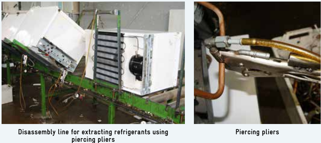
Figure 14: Disassembly line for extracting refrigerants and the associated piercing pliers
