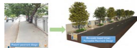
One of the possible design interventions for urban greening and stormwater management. Source: Care Earth Trust
