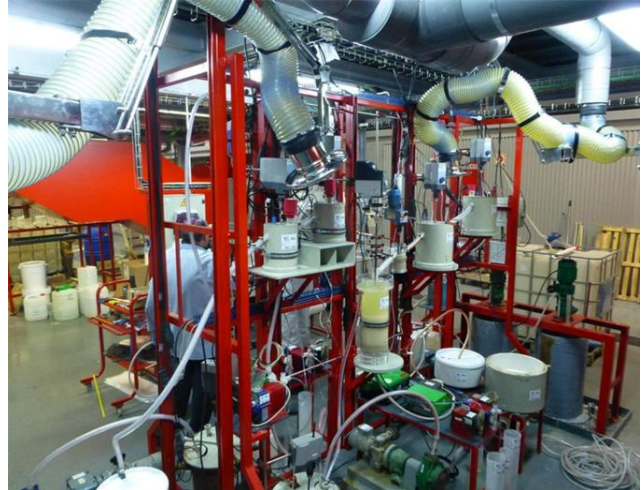
Figure 41: Example of a rare earth recovery plant (pilot) (Reclite SA (Pty) Ltd 2019)
