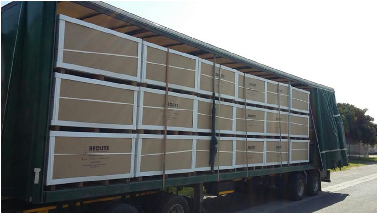
Figure 61: Sample transport truck with transport containers for hazardous products made from recyclable cardboard; maximising volume on long distance trucks (Reclite SA (Pty) Ltd 2019)
