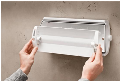
Figure 3: Manual dismantling of luminaires (Reclite SA (Pty) Ltd 2019)
