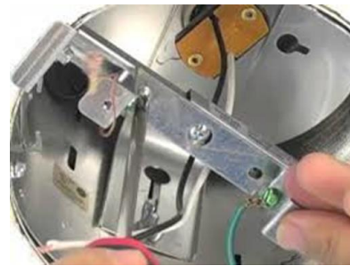
Figure 4: Manual dismantling of luminaires (Reclite SA (Pty) Ltd 2019)
