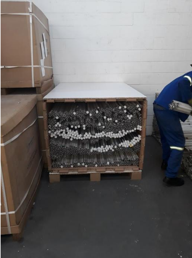
Figure 63: High-volume transportation container with linear waste lighting tubes. (Reclite SA (Pty) Ltd 2019)
