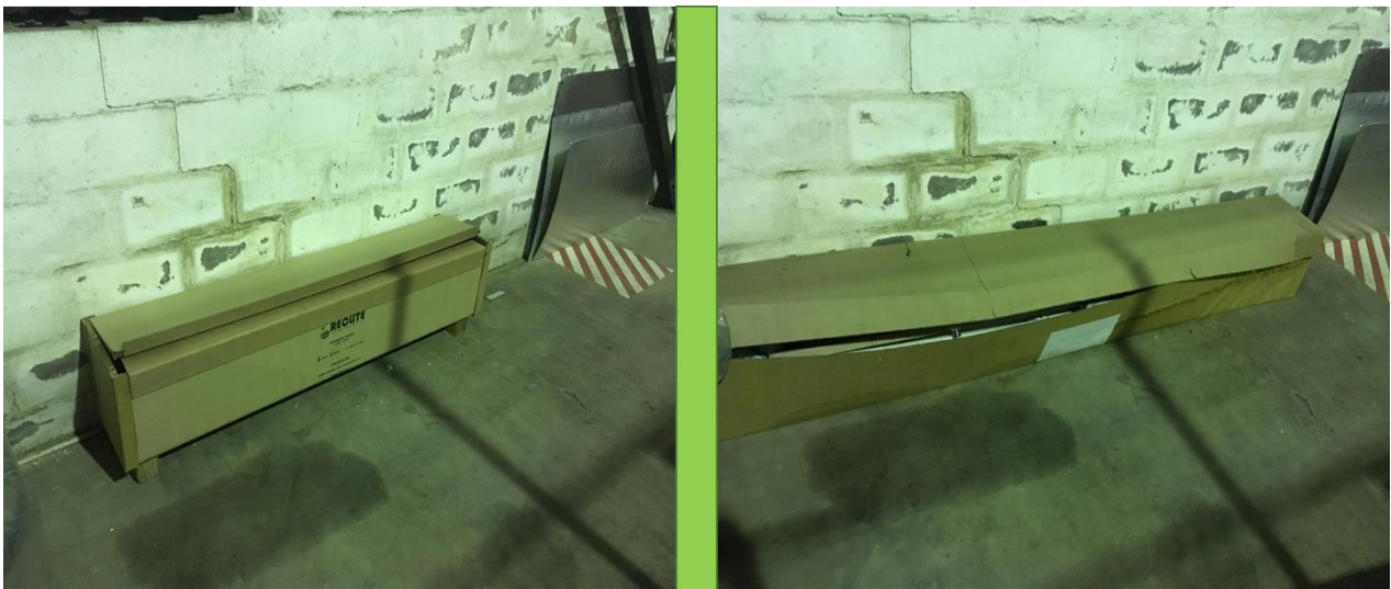
Figure 53: Comparison in design of small volume containers in a warehouse for spent lamp collection (left correct / right incorrect). The badly designed container on the right collapses and is prone to moisture absorption from the floor as it is not off the ground (Reclite SA (Pty) Ltd 2019)
