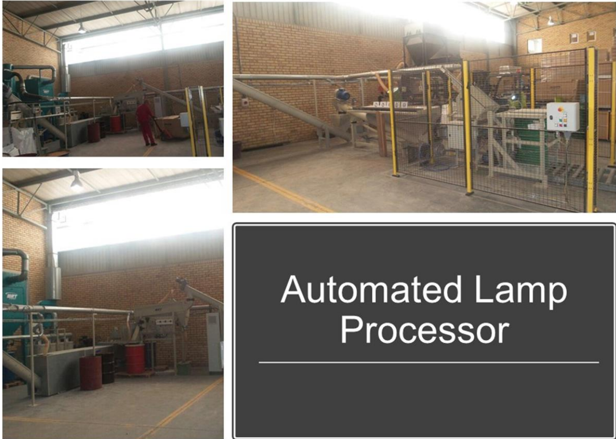
Figure 29: Swedish dry technology machinery type LP600 at Reclite SA in South Africa (Reclite SA (Pty) Ltd 2019)
