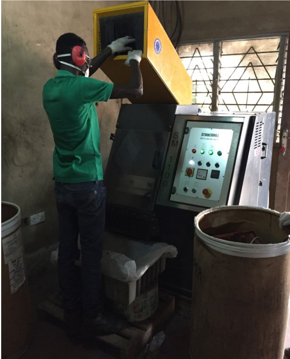
Figure 6.8: Granulation of Cu- and Al-cables at City Waste Recycling
