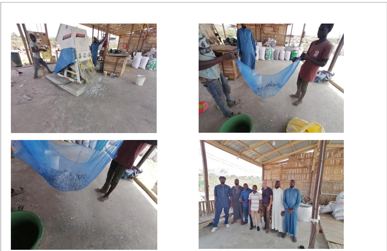
Figure 5-15: Shredding and sieving of HIPS at the “plastics hotspot”
