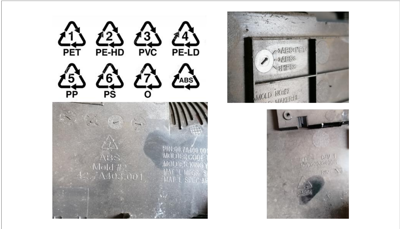
Figure 4-4: Sorting according to label: labels and typical labelling on back of appliance
