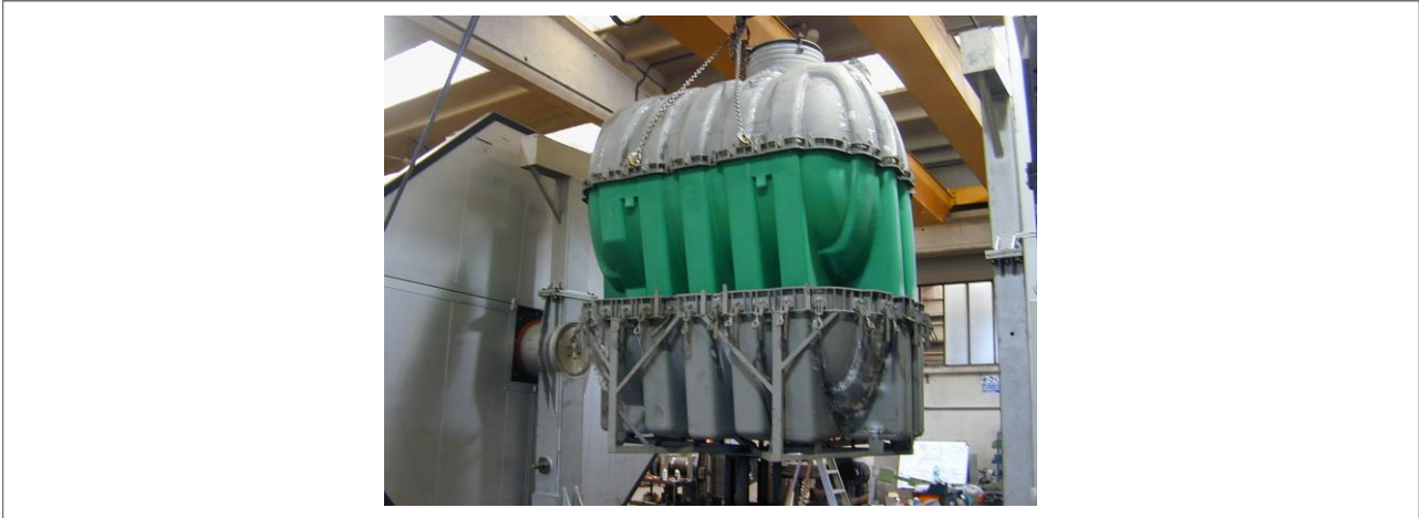
Figure 3-12: Processing method 8: rotational moulding
