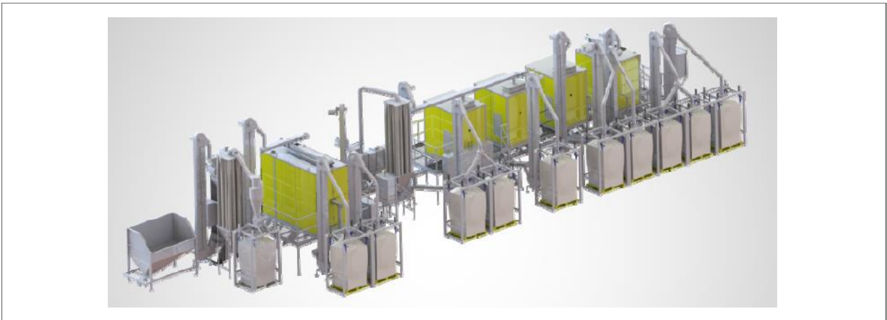
Figure 5-11: “Machine route”: state of the art WEEE plastics recycling plant
