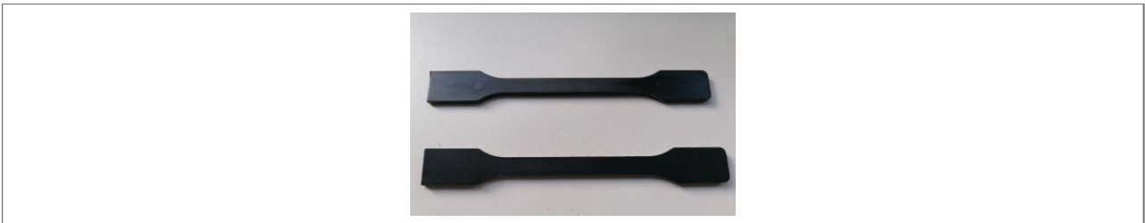
Figure 5-20: Tensile bars made by injection moulding at TITK for ABS 001
