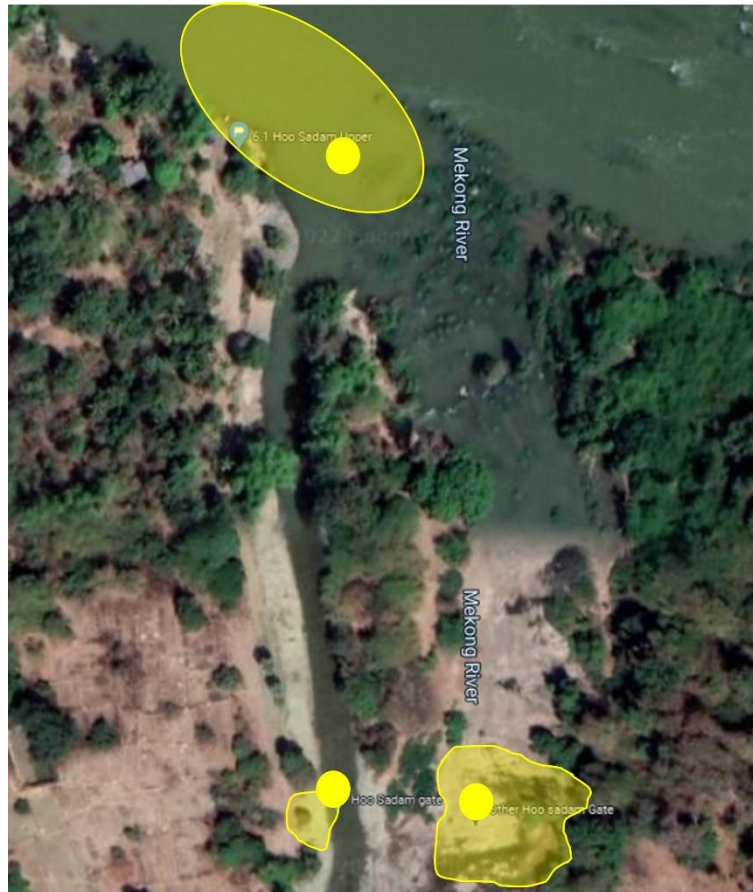
Plate 17. Three receivers were placed at the top of Hoo Sadam. The top receiver had a known good range because of engineering to increase depth and level the substrate. It would perform well in the wet and dry seasons. The lower two receivers only targeted upstream migrating fish and were positioned near resting pools and gaps in the vegetation. In the wet season the water in the channel to the right of the photo is up to 1.5 m deep and it is possible for fish to exit at the top without hitting the top receiver. In the dry season, all fish must enter or exit within 20 m of the top receiver, but the other two receivers are out of the water.
