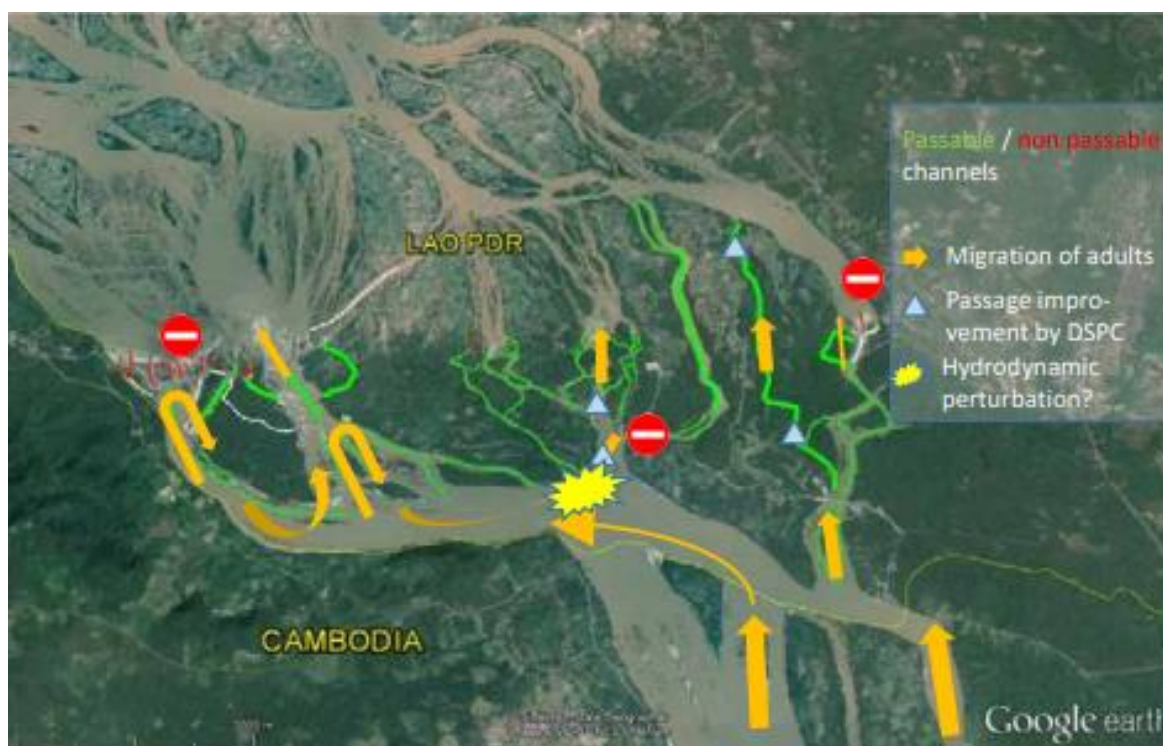
Figure 2. Synthesis representation of passage, migrations and obstacles at Khone Falls. The green represents flow and the orange represents fish movement patterns (source: MRC 2020). The thickness of the arrows represents volumes of fish using that route. Anecdotal comments on this diagram following the results of this study are included in Appendix A.
