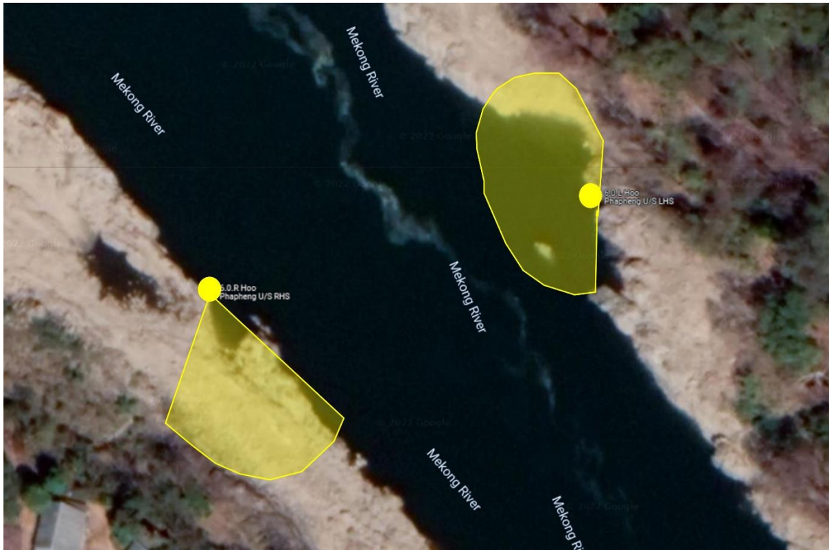
Plate 16. Use of slower water areas in Hoo Phapheng to give greater detection probability of fish migrating upstream. In this case, the centre of the channel is very fast flowing and detection is not covered. Nevertheless, most fish will stay near the edges and use the resting pools where the receivers are located. The pools also align with gaps in the vegetation to aid in detectability.
