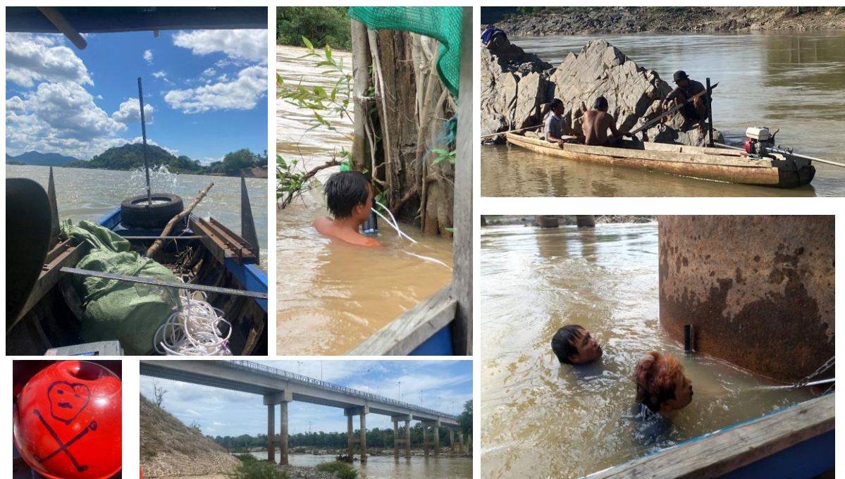
Plate 11. Methods used to deploy the receivers included attaching them to existing structures or rocky outcrops in channels or using an anchor and receiver tower structure in the Mekong mainstem.
