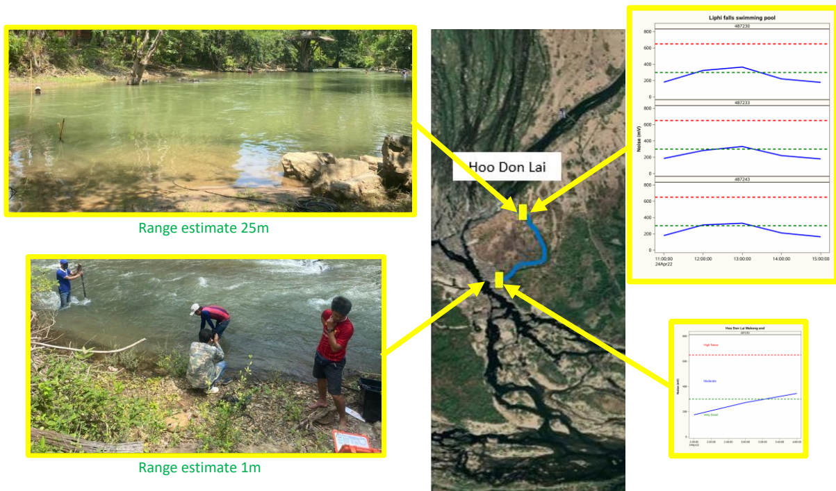
Figure A1. Range tests in Hoo Don Lai in April of 2022. Graphs are background noise levels and values below the green reference line are desirable.
