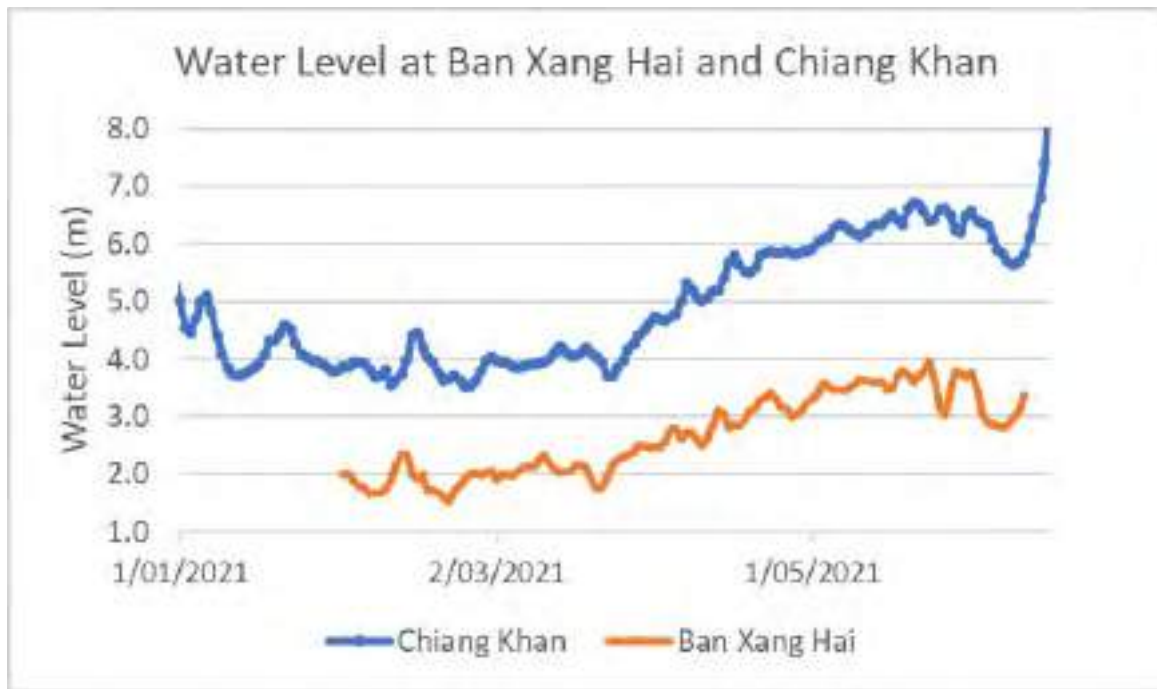
Figure 3-4. Comparison of water level measurements at Ban Xang Hai and Chiang Khan.
