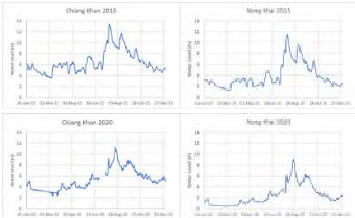
Figure 2.8. Water level at Chiang Khan and Nong Khai in 2015 and 2020 based on 15-minute recordings at HYCOS sites.
