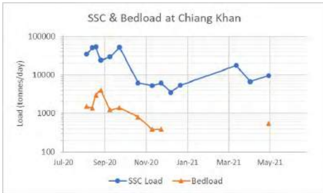
Figure 3-15. Comparison of SSC load and estimated bedload at Chiang Khan from July 2020 to Jun 2021.
