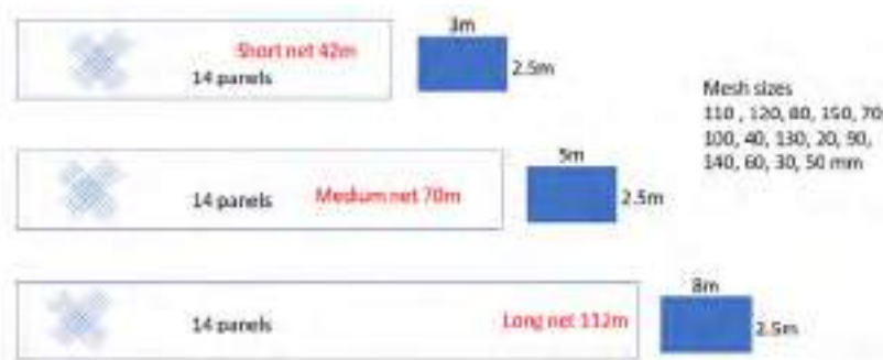
Figure 5.2. Dimensions of gillnet sets tested
