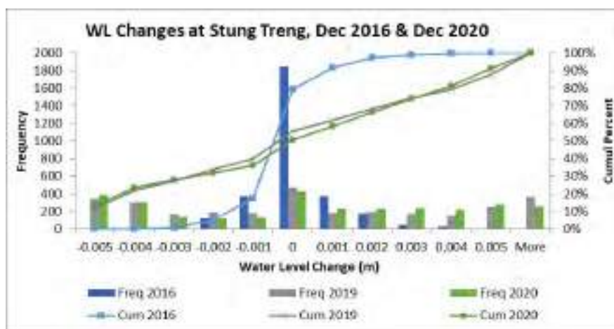
Figure 2.6. Histogram and cumulative percent of water level changes at Stung Treng in December 2016, 2019 and 2020
