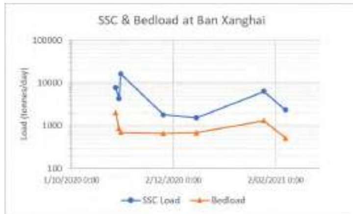
Figure 2.34. Comparison of SSC load and estimated bedload transport at Ban Xanghai, October 2020 – February 2021
