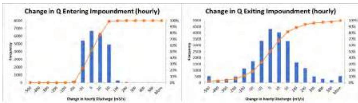
Figure 5-10. (left) Hourly changes in flow rate entering the impoundment and (right) discharged from the Xayaburi HPP. Data provided by the operator of Xayaburi.
